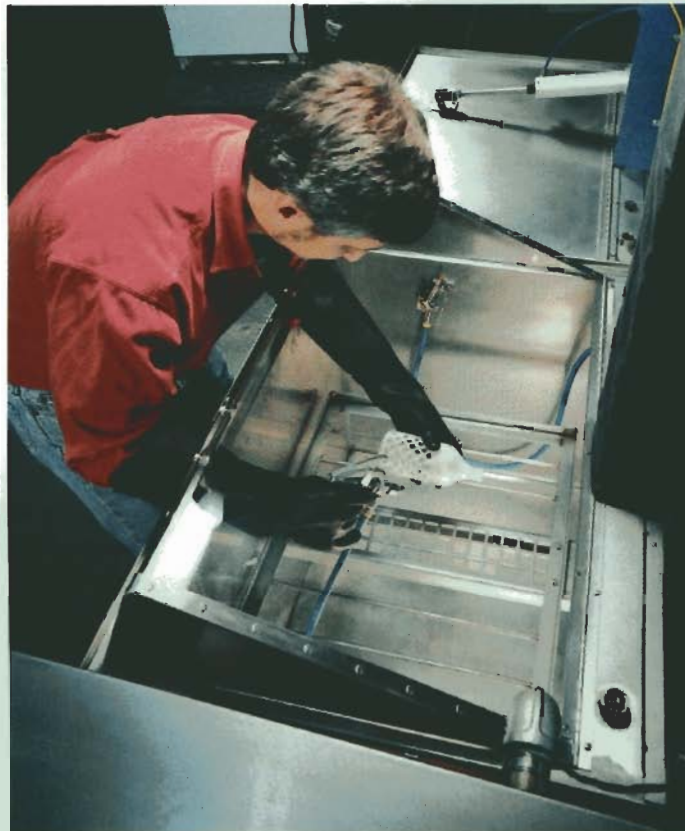
The Rinse Station includes a lexan lid with built in rubber gloves.
